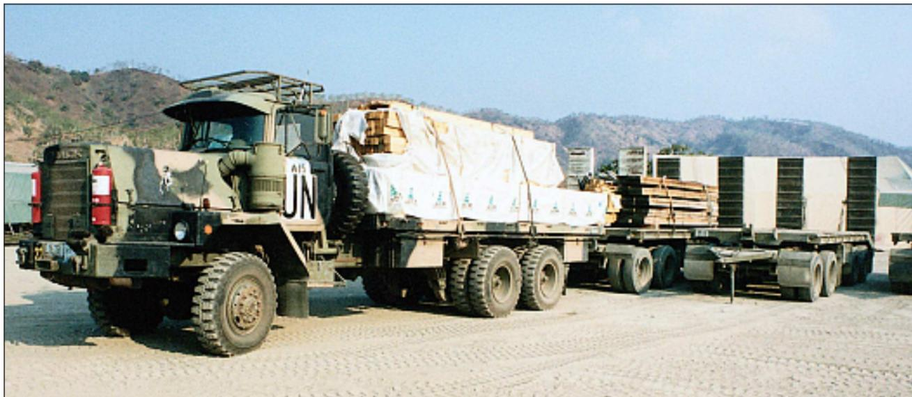
Truck, Cargo, Heavy, MC3 with winch, laden with timber and coupled to a 20-tonne plant trailer (Ron Fry)
